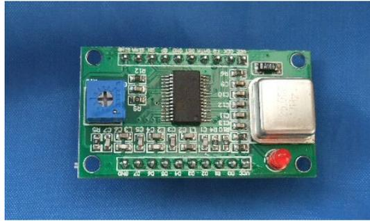
Figure 8.4 DDS Module (pre-assembled)
