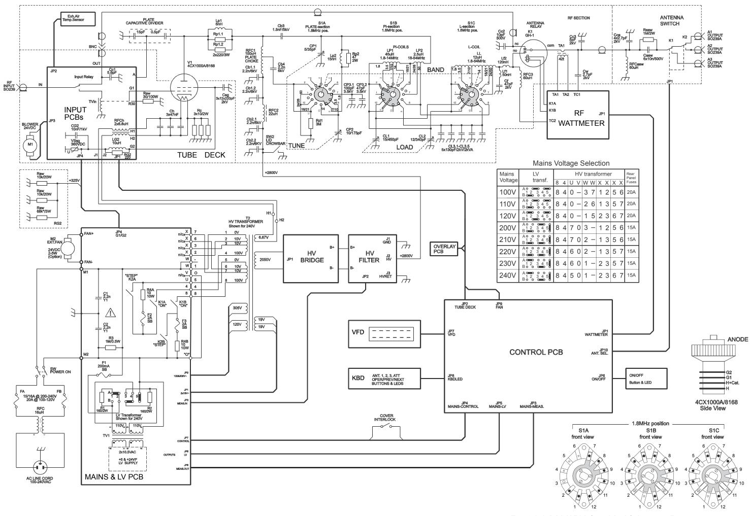
Fig. 6.1 ACOM1500 Simplified Schematic Diagram
