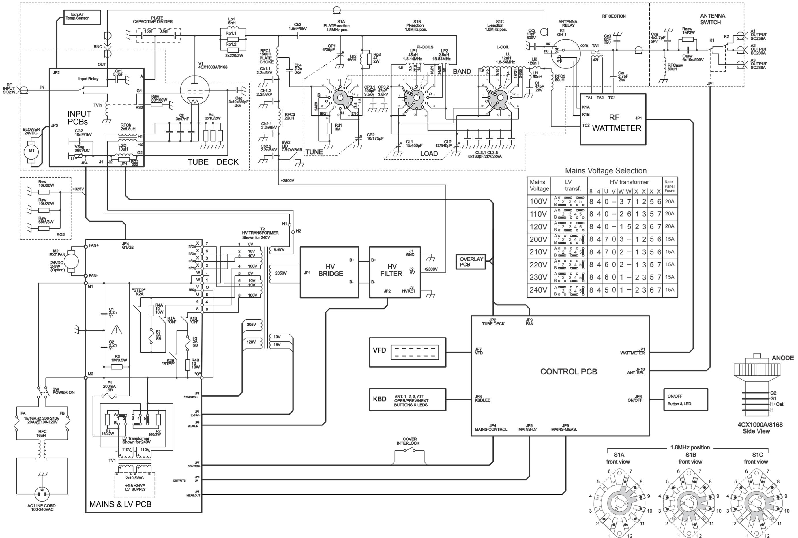
Fig. 6.1 ACOM1500 Simplified Schematic Diagram
