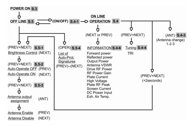
Fig.3-2 Information Screens and Control Functions Structure
